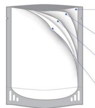
POLYPROPYLENE Physical Food Contact Layer • Heat Seal Surface • Provides Flexibility and Strength
